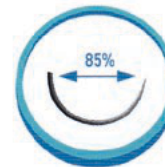
Needle Compressed to 85% of its chord length. La aguja se comprime hasta el 85% del ancho del hilo
